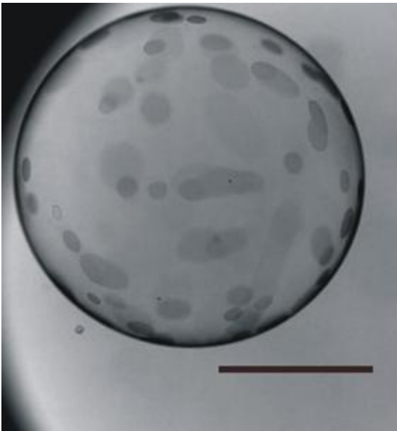
As the reason for the delayed dynamics in the second phase of the soap bubble relaxation, we identify dislocation dynamics and the surface reduction by island formation. The dark spots on the bubble are islands of excess smectic layers that have formed during the relaxation [May2012].
