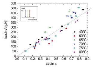
Stress vs strain curves of 30 micron thick smectic elastomer fibers at different temperatures [Stannarius2012]
