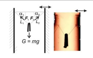
Measurement of tensions by means of a load attached to a vertically suspended smectic fiber
