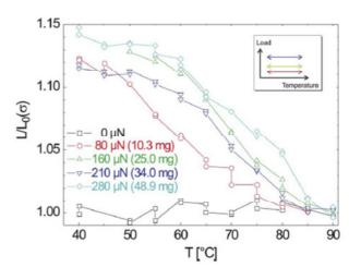
Length changes of the filament with attached weights at cooling from the isotropic phase down to room temperature [Stannarius2012] R. Stannarius, H. Schüring, C. Tolksdorf, and R. Zentel. Elastic properties of liquid crystal elastomer balloons. *Mol. Cryst. Liq. Cryst.*, **364**, 305 (2001).
