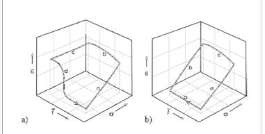
Thermo-elastic behaviour in the temperature-stressstrain diagram. When the parameter changes in the  $\sigma$ -T plane are clockwise, we find shape memory effects, when the parameter variation is counterclockwise, the material behaves normally [Stannarius2012].
