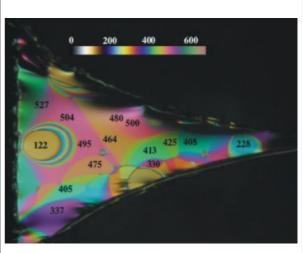
Color changes of the film show that the film of a diluted copolymer becomes thinner with increasing strain. It behaves similar to an isotropic rubber with Poisson ratio 1/2. The three following images show the same smectic A elastomer film at elongations  $x/x_0 = 1.34$ , 1.60 and 1.90.
