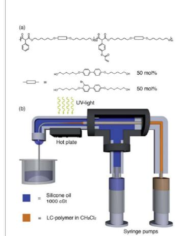
Setup for the preparation of smectic main chain elastomer fibers by means of a wetspinning technique [Ohm2011]
