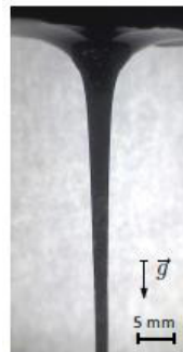
Meniscus of a ferrofluid around a wire carrying a current of 70 A. The ferrofluid is embedded in a liquid of higher density (glycerol/water mixture)
