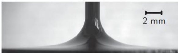
The image shows the meniscus around a wire carrying 70 A.
